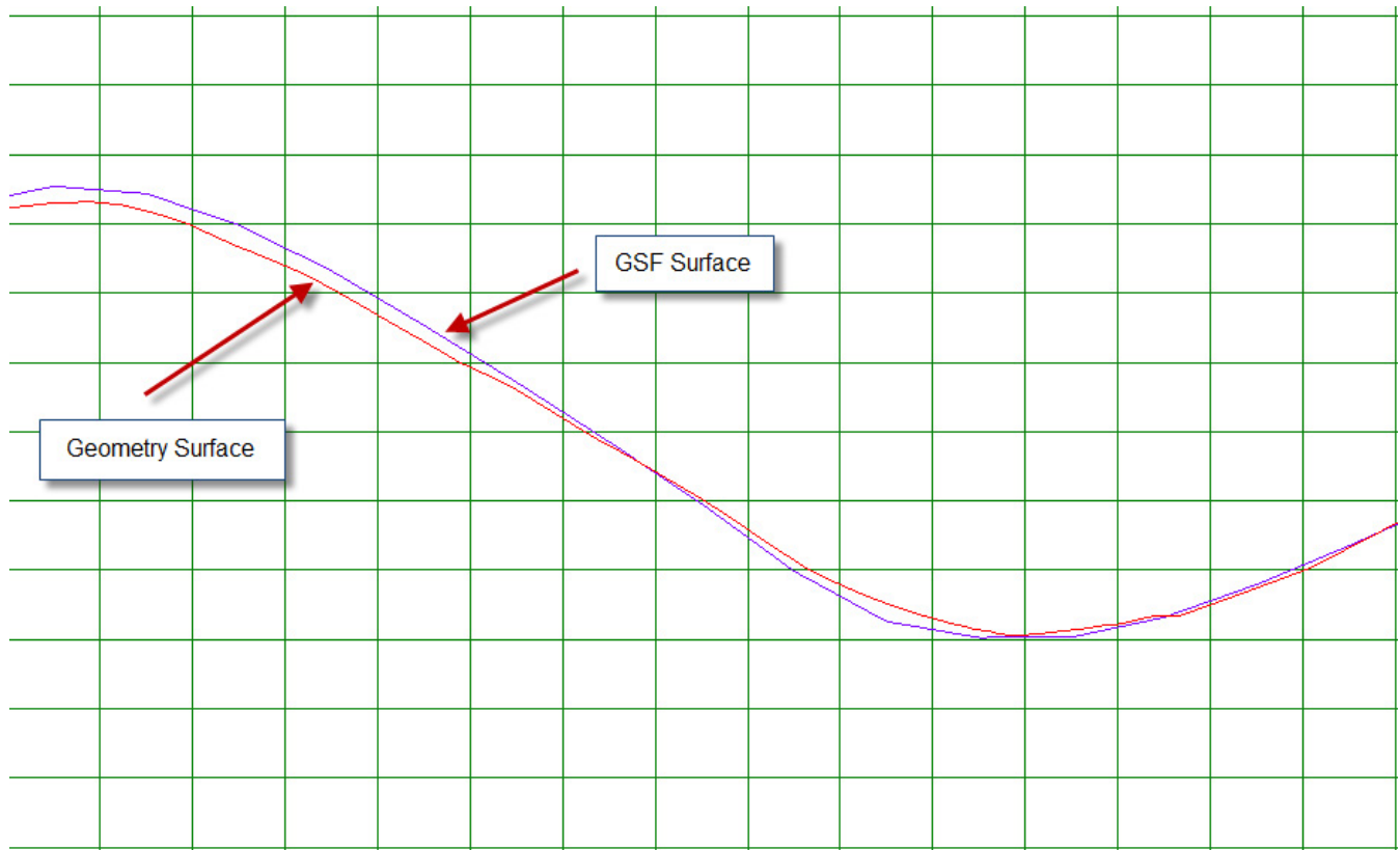
Figure 1: This sectional view indicates the differences that can be observed when viewing GSF surfaces that are a product of gridded geometry surfaces in 2D.
