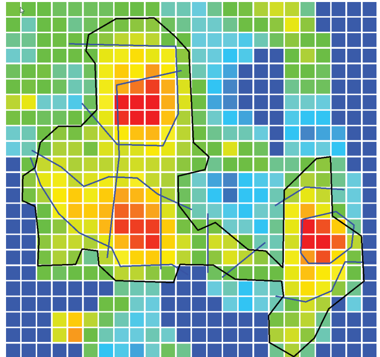
Figure 3. The black polygon encompasses the higher grade material. The blue polylines and polygons divide the material based on grade and material destination requirements.
